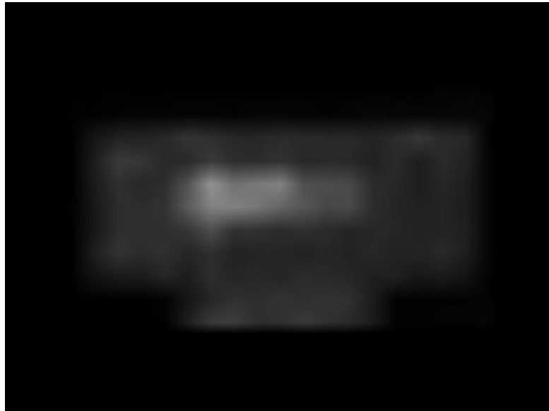
Figure 5. Neutron diffraction image of d\sim 1.15 \text{ \AA} peak, corresponding to 211 reflection of the BCC SUS430 measured at NOVA.
