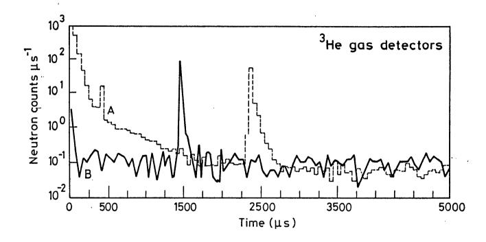
Figure 2 Comparison of time-of-flight scattering data from vanadium taken without (A) the chopper and with (B) the chopper. For clarity two different incident energies ( A : 220 meV and B: 600 meV) are shown. The background effect is independent of the choice of fast chopper energy.
