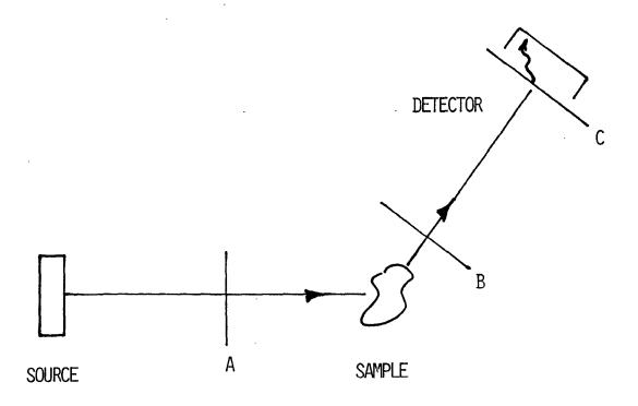
Fig. 1 Schematic diagram of Electron Volt Spectrometers.
